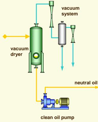
Residual moisture is removed by a dryer under a vacuum of < 50 mbar.
