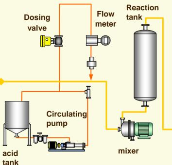
The acid is circulated with a certain pressure by a circulating pump.
