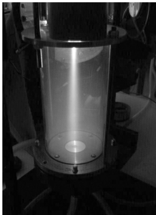
Fig. 2 Image of a low-pressure nitrogen plasma beam (100 W, 2 mbar).
