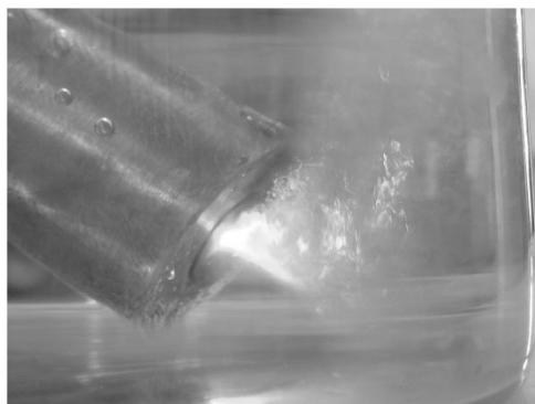
Fig. 9 Underwater operation of over-atmospheric-pressure RF-jet.
