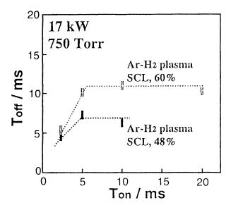
Fig. 8 Limitation of the pulse modulated operation of induction thermal plasma.
