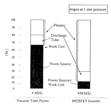
Fig. 9 Power dissipation in plasma generation for MOSFET transistor system (after Sakakibara et al. [8]).
