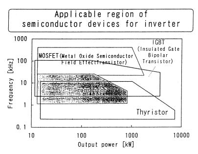
Fig. 1 Applicable region of power transistor.
