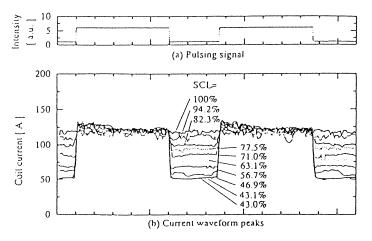
Fig. 4 Pulse modulated coil current.
