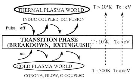
Fig. 10 Concept of pulsation in cold and thermal plasmas.
