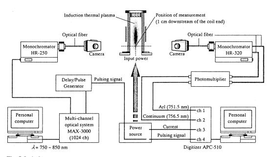
Fig. 5 Optical measurement system.
