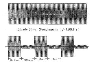
Fig. 2 Principle of pulse modulating.
