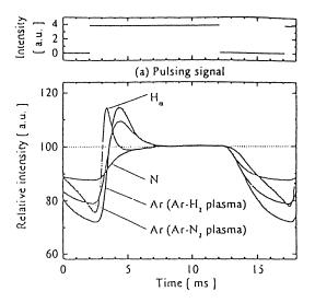
Fig. 7 Time evolution of emissions from Ar, N and H.
