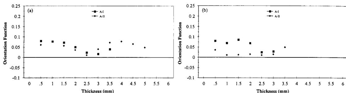
Figure 6. The Hermans orientation functions of the 040-reflection  $f_{040,ND}$  with respect to ND as a function of the distance  $d$  from the surface of the plaque. a) PP/ g 5 STATIC, b) PP/ g 10 STATIC (refer to Fig. 2 for sample location ).
