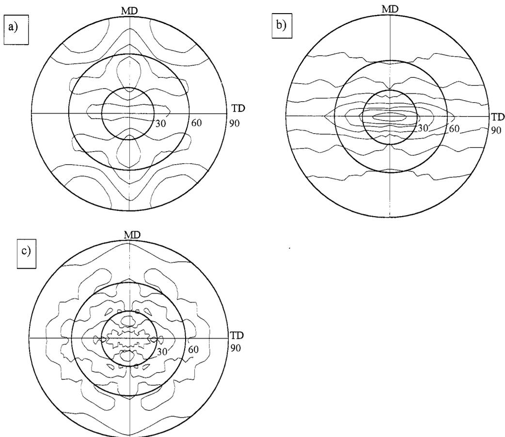
Figure 4. An example of the pole figures from the a) 110-, b) 040-, and c) 130- reflections of polypropylene from the layer at 2 mm depth in sample **PP/g 5 STATIC**.
