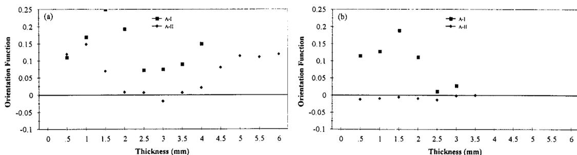
Figure 5. Hermans orientation functions of the chains  $f_c$  with respect to MD as a function of the distance  $d$  from the surface of the plaque. a) **PP/g 5 STATIC** b) **PP/g 10 STATIC** (refer to Fig. 2 for sample location).
