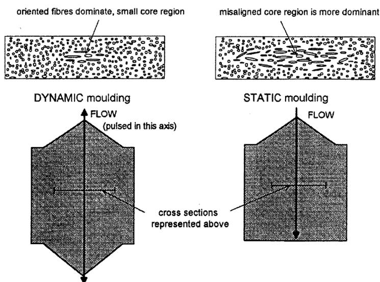
Figure 8. A schematic representation of the two moulded parts and the fiber orientation in the central section shown.
