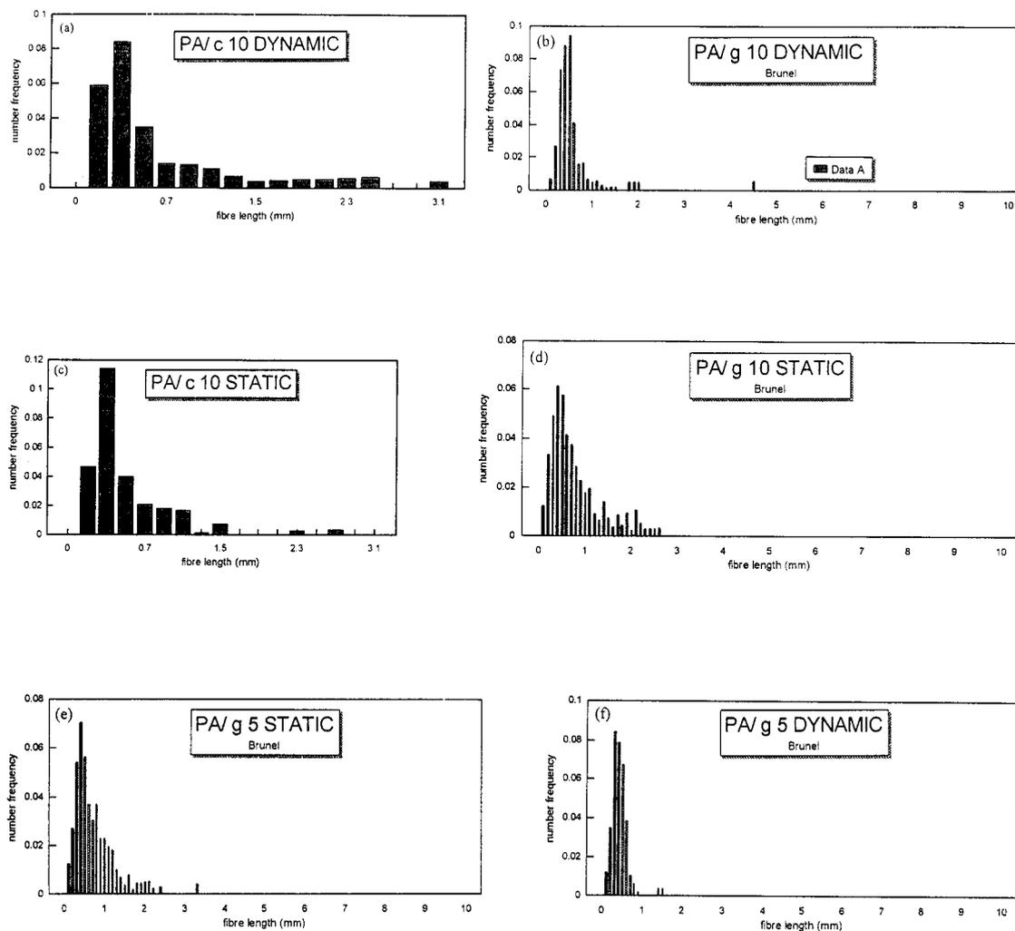
Figure 11. (a - f) Fiber length distributions plotted for polyamide composites (Laboratory 6). The carbon fiber materials are shown with a different fiber length axis. It is clear that the dynamic moulding technique reduces the fiber length statistics compared to the conventionally moulded static process.
