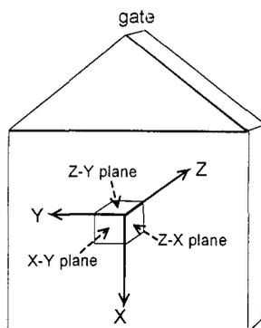
Figure 9. Definition of planes for the characterisation of the 3D fiber orientation functions
