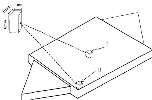
Figure 2. A schematic diagram showing the location of the rods extracted from the middle (I) and edge (II) of the sample.
