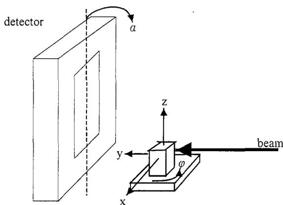
Figure 3. The experimental set-up of the rod in the beam. The rod is moved in the z-direction to measure the pole figures of different locations in the sample. The detector is turned around the y-axis and the sample is turned around the x-axis.
