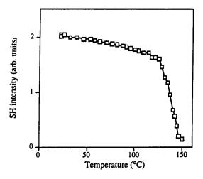
Figure 1. Second harmonic intensity from spin coated film of poly(BPOD) at various temperatures.
