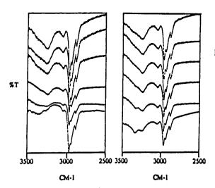
Figure 2. FT-IR spectra of spin cast films of poly(BPOD) in 2500-3500 cm-1 region.
