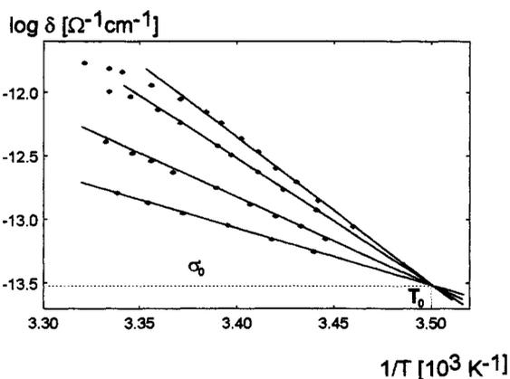
Fig. 12. Semiconductivity data for 15,15'-*cis*- $\beta$ -carotene powder cell with the absorption of different amounts of ethyl acetate vapour (ref.25).
