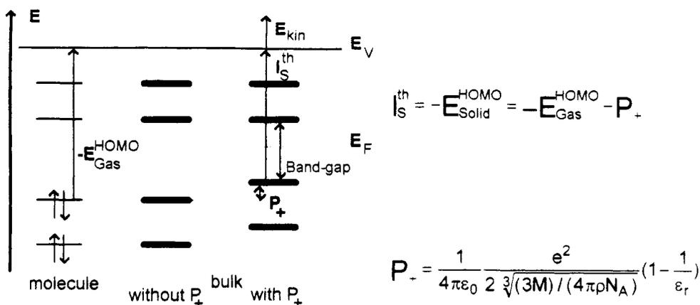
Fig. 8. Illustration of the energy levels
