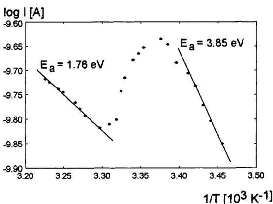
Fig. 11 Semiconductivity in an ethyl acetate powder cell of 15,15'-*cis*- $\beta$ -carotene as a function of temperature (ref. 25).
