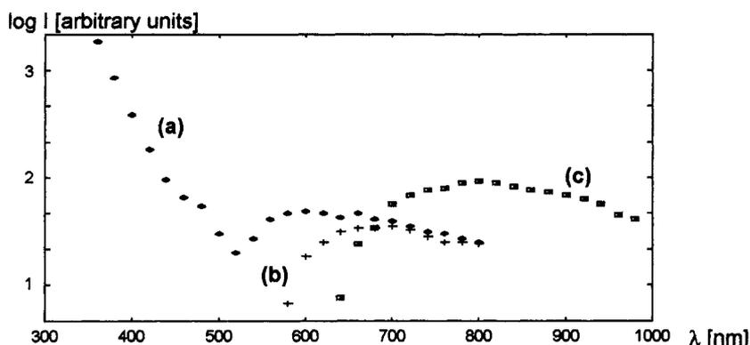
Fig. 10. Photoconductivity spectra of  $\beta$ -carotene sandwich-type cell (Cr/Car/Cr) and surface type sample. (a) Spectra when positive electrode is illuminated, (b) spectra when negative electrode is illuminated, (c) surface-type sample spectra (ref. 19).
