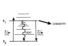
Figure 3. Events that may occur after a molecule is excited: emission of light (hv), release of heat (wavy line) and chemistry (heavy arrow).
