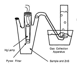
Figure 7. A schematic of a photochemical reactor for irradiation of ZnS suspensions and collection of gases produced.
