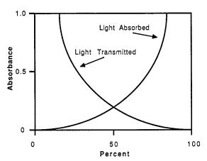
Figure 2. Relationship between the absorbance and the percentages of light intensity absorbed  $(I_a/I_0)$  and transmitted  $(I_t/I_0)$ .
