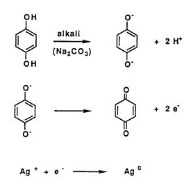
The reduction of Ag<sup>+</sup> does not progress without the latent image. The quantum yield of latent image formation is less than unity, though the redox development reaction amplifies the final imaging yield, and the reduced Ag forms a black image. Hydroquinone is not dissociated under acidic condition, and so acetic acid is effective in stopping the development.
