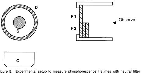
Figure 5. Experimental setup to measure phosphorescence lifetimes with neutral filter sets: C = camera flash; S = sample; D = Dewar vessel; F1 and F2 = filter sets.
