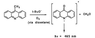
The apparent first-order rate constant at  $40^{\circ}$  C is 1.0 min<sup>-1</sup>, the activation energy is 65 kJ mol<sup>-1</sup>, the chemiluminescence quantum yield is  $6.3 \times 10^{-3}$ , and the peak of the emission is at 465 nm (fluorescence from the acridone anion).
