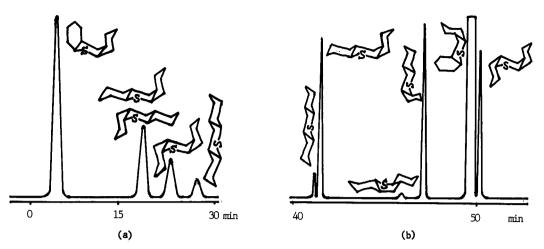
Fig. 1. Chromatogram of PHTX: (a) GTCB, 2m x 1mm, temperature programming 200° to 280°C, 10/min; (b) SP-1000, 50 m x 0.25 mm, temperature 145°C.
