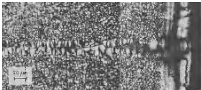
Fig. 14 Polarised light micrograph taken by BP, showing the weld region in a section from a Type I PA66 plaque.
