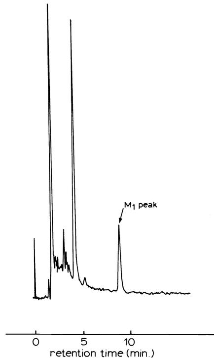
Fig. 10.  $C_{18}$  reverse phase HPLC chromatogram of an extract of milk powder, containing ca. 0.4  $\mu\text{g } M_1/\text{kg}$ , prepared according to the method of Stubblefield (ref. 35) by Mulders (ref. 36)
