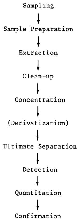
Fig. 2. Analytical procedure for mycotoxin determination
