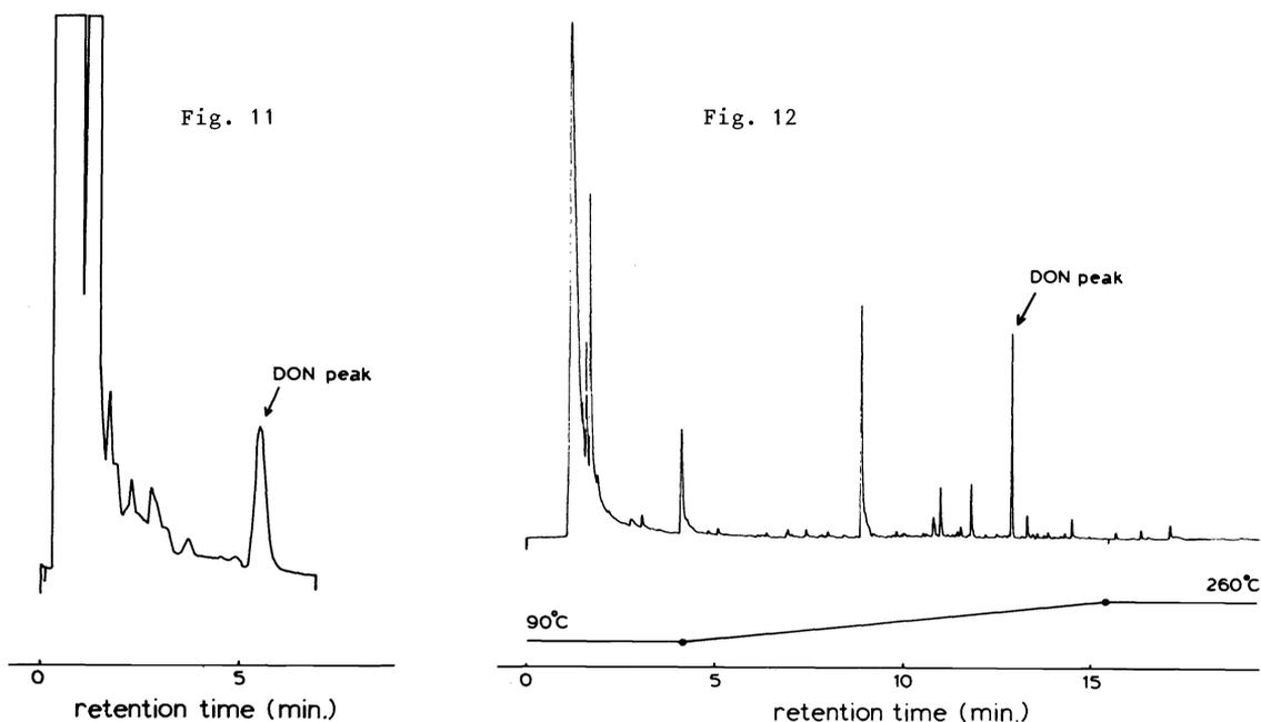
Fig. 11. GLC chromatogram (3% OV-3) of an extract of maize, containing *ca.* 60  $\mu\text{g}$  deoxynivalenol/kg, prepared according to the modified method of Scott (ref. 41) by Besling (ref. 42)
