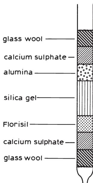
Fig. 3. Packing of a minicolumn according to Romer (ref. 12)
