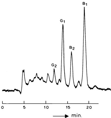
Fig. 9.  $C_{18}$  reverse phase HPLC chromatogram of an extract of feedingstuff containing citrus pulp, contaminated with aflatoxins  $B_1$ ,  $B_2$ ,  $G_1$  and  $G_2$  at ca. 12, 3, 8 and 1  $\mu\text{g}/\text{kg}$  respectively, prepared according to the method of Van Egmond (ref. 34)
