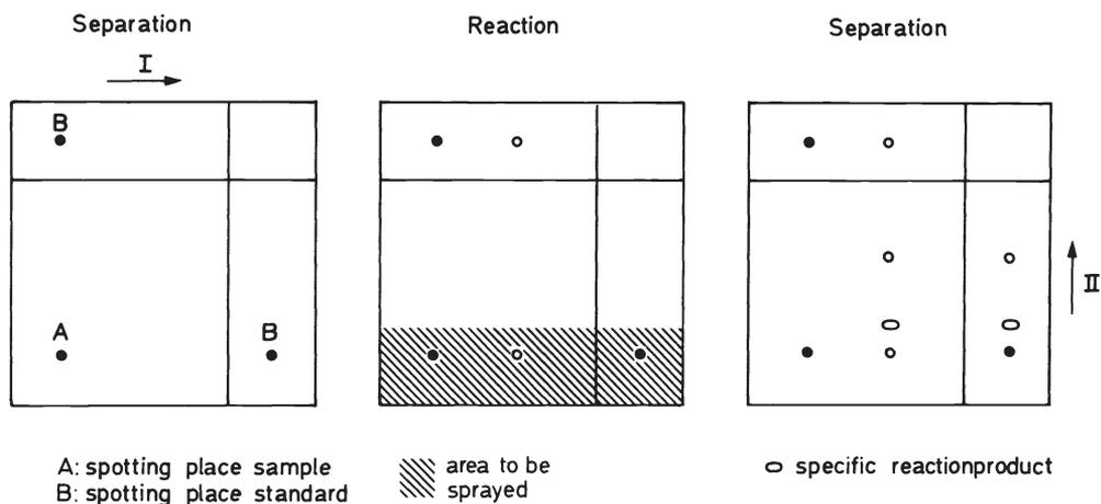
Fig. 7. Schematic representation of the two-dimensional TLC confirmatory test of Verhülsonk (ref. 24)
