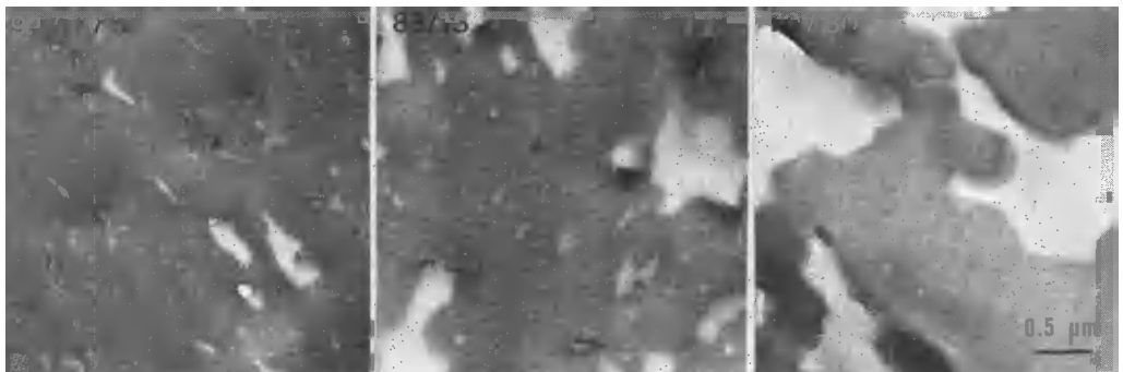
Fig.37. Electron micrographs of PVC/PVA blends of different composition, milled at 160 and 180°C; ref.(39).
