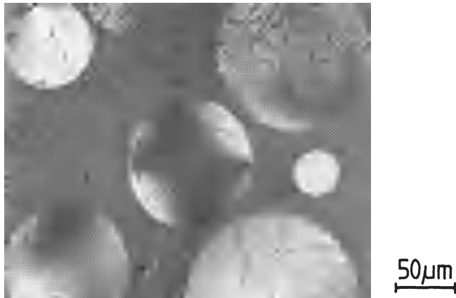
Fig. 13. Anisotropic mesophase, formed in isotropic petrol pitch by heat treatment at 400 °C.
