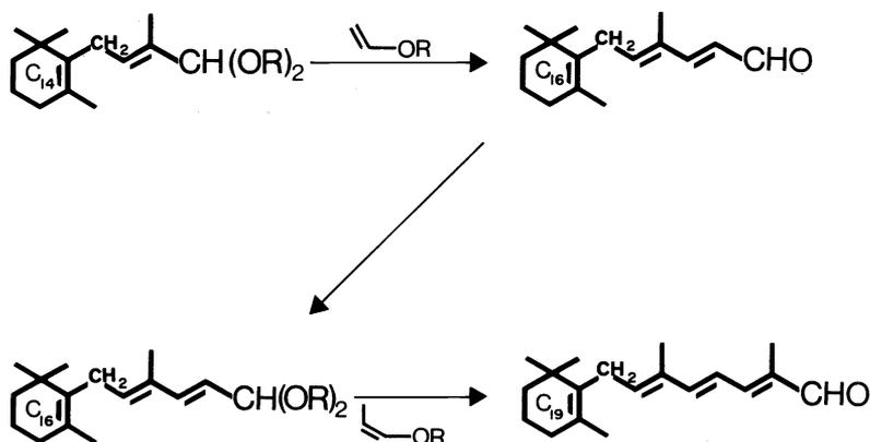
Fig. 14. Lengthening of  $\beta$ - $C_{14}$ -aldehyde to  $\beta$ - $C_{19}$ -aldehyde
