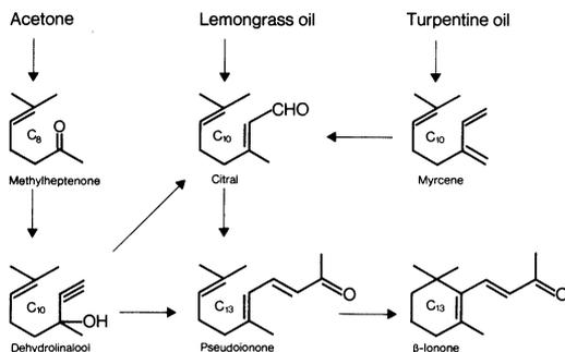
Fig. 2. Manufacture of  $\beta$ -ionone from various sources
