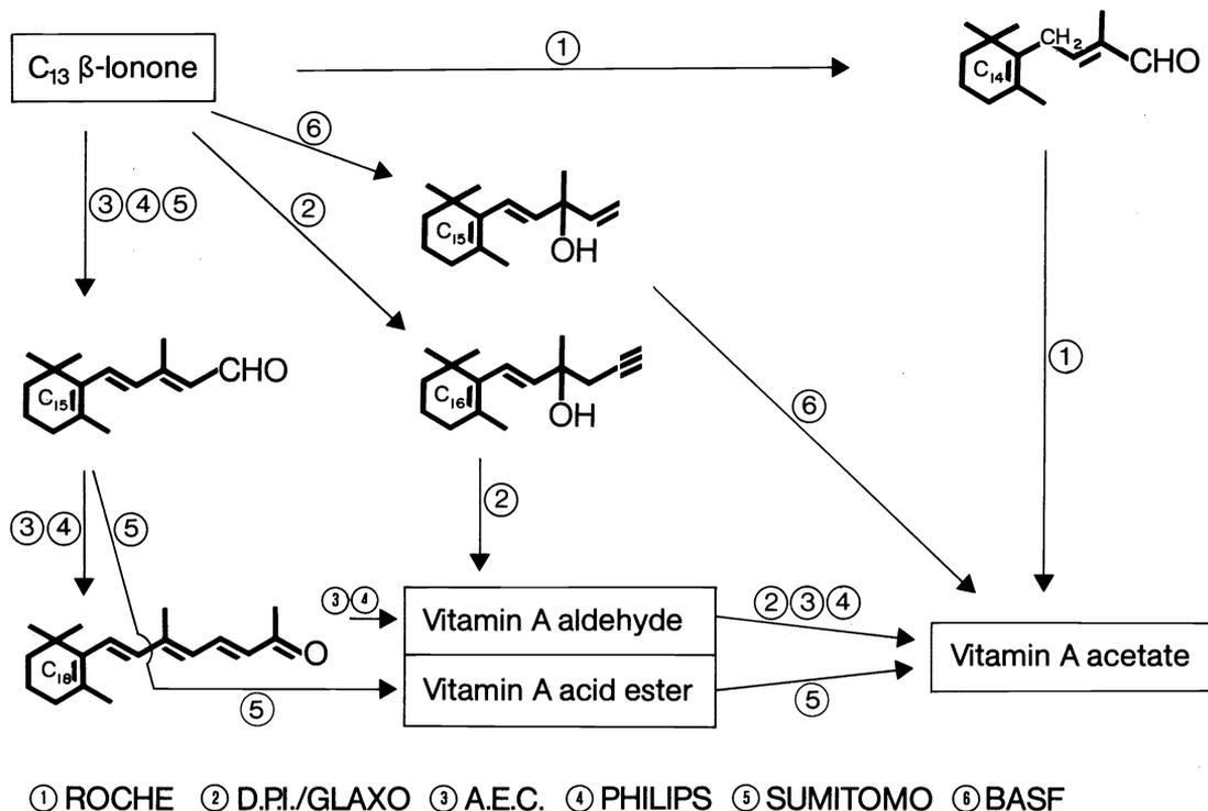
Fig. 10. Key intermediates of vitamin A manufacture
