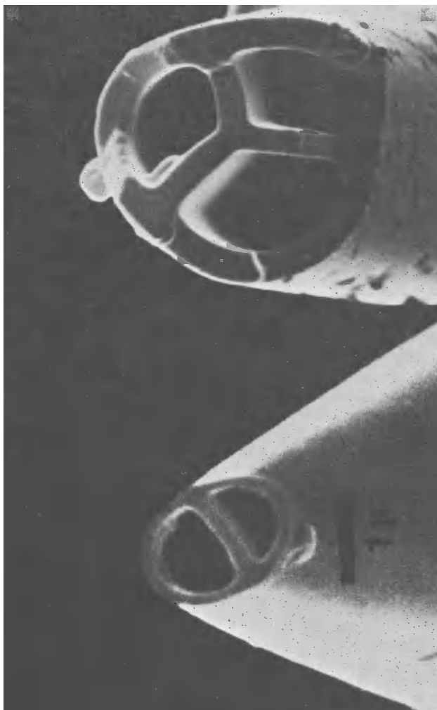
Figure 6. Scanning electron microscope view of multichannel microelectrode tips (see also ref. 45). (Courtesy of Mr. D. Schäfer and Mr. K. Zierold).
