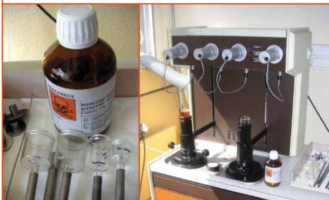
**Intruding mercury up to 400 MPa allows for the determination of pore width, from 3 nm to 100  $\mu\text{m}$ , in rigid porous materials. The glass intrusion chamber (four different sample sizes are shown here) is to be filled with the sample and then with mercury before being inserted in the high pressure unit (here accommodating two chambers). After each experiment, the mercury spoiled with powder and oil (used to exert the pressure) needs to be cleaned and distilled.**
